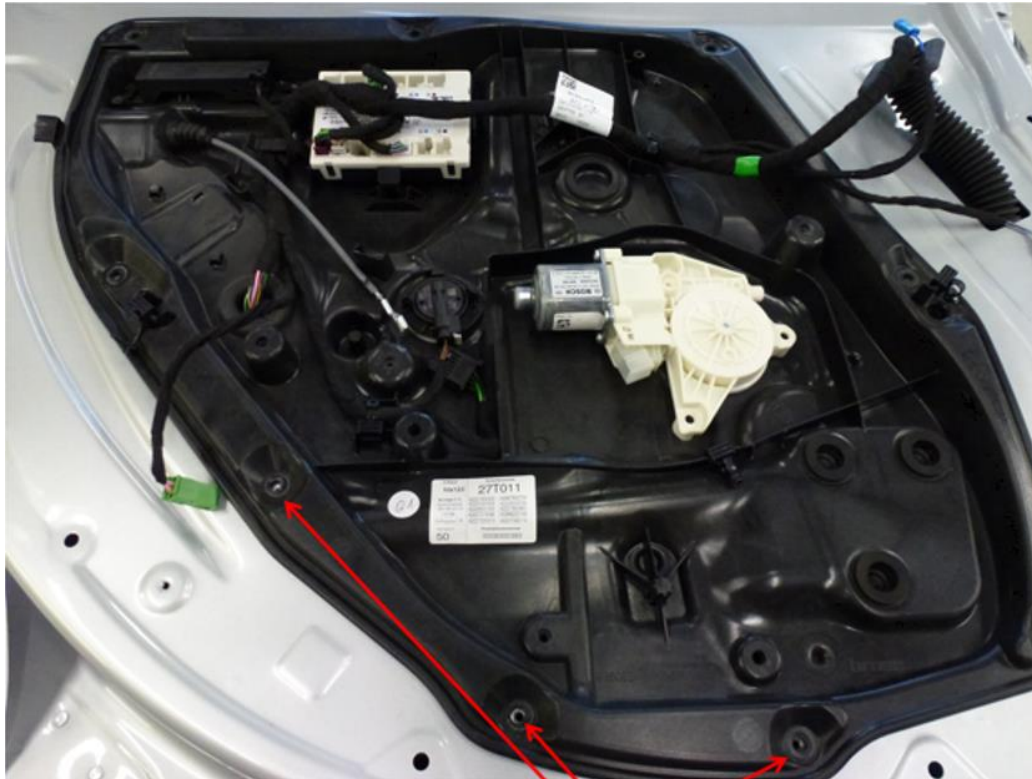
aligned holes of door and module ready for screwing
