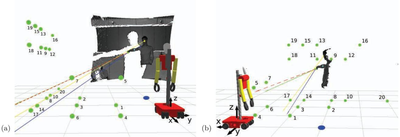
**Figure 4: Illustration of experiment setup from (a) frontal and (b) side view. The test person stands in front of the robot at 2 m distance (blue dot) and points to the pointing targets (green spheres). Estimated pointing directions are depicted by arrows: head-hand (blue), elbow-hand (dashed red), shoulder-hand (black), and GPR (yellow). The robot measures angles between body features in its base coordinate frame (black).**
