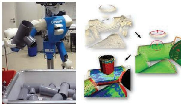
**Fig. 1.** Left: Robot grasping a found pipe object out of a box. Right: we detect 2D contour and 3D shape primitives in 3D point clouds and perform graph-matching to detect objects and to estimate their pose.
