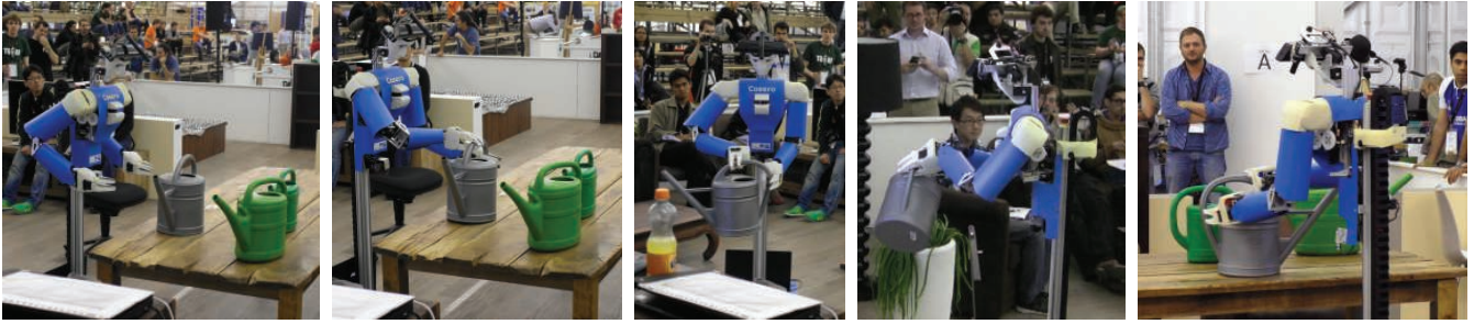
Fig. 5. Cognitive service robot Cosero manipulates a novel watering can during the Open Challenge at RoboCup 2013 in Eindhoven, Netherlands. We specified bimanual grasp poses, the can’s end-effector, and the motion of the end-effector for watering a plant for another watering can instance. Cosero used our deformable registration method to efficiently align the can in its current RGB-D image with the model can. From the displacement field Cosero estimates the poses of the grasps and the watering can’s end-effector using our proposed local transformation estimation method. It then grasps the watering can and waters a plant using the generalized skill.
