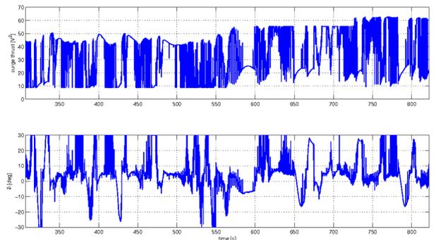
Fig. 7. Commanded signal on thrust motors (upper plot) and rudder (lower plot).
