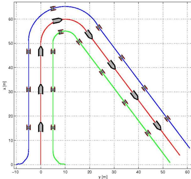
Fig. 8. Simulated vehicle formation trial. One simulated ALANIS (red line) as *leader* vehicle, two simulated Charlie (blue and green lines) as *follower* vehicles.
