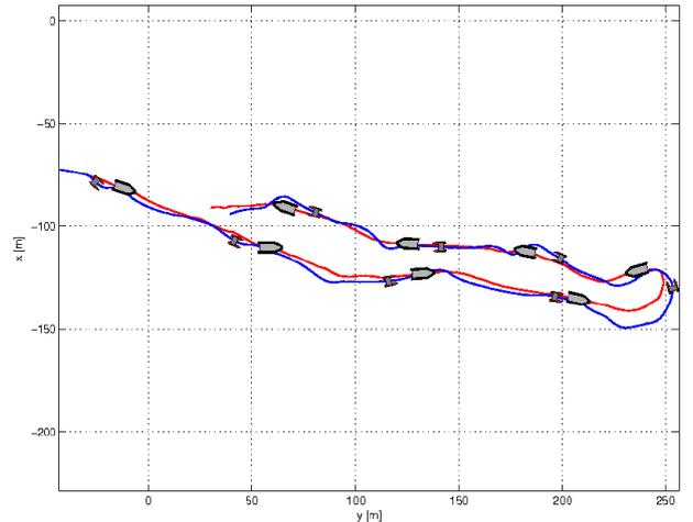
Fig. 5. Experimental vehicle-following trial. ALANIS (red line) as *leader* vehicle, Charlie (blue line) as *follower* vehicle.
