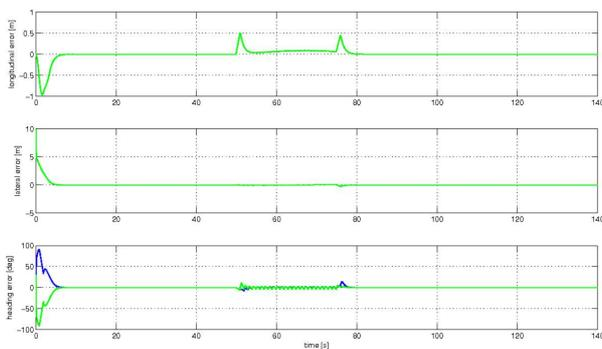
Fig. 9. Simulated vehicle formation trial. Lateral, longitudinal and orientation errors, green line - *follower-1*, blue line - *follower-2*
