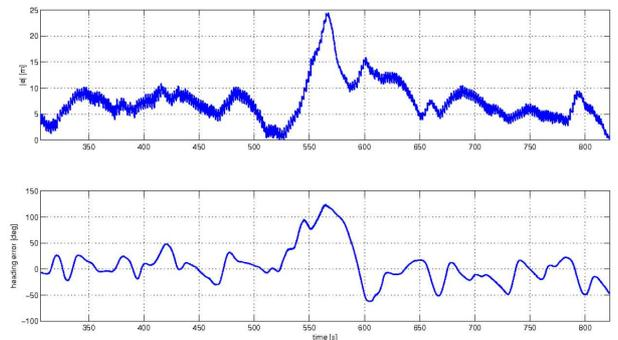
Fig. 6. Experimental vehicle-following trial. Absolute value of the position error (upper plot) and orientation error (lower plot).
