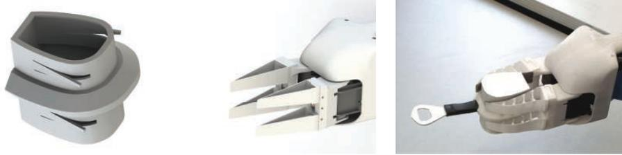
**Fig. 3.** Tool Adapters. We designed special adapters for tools to establish stable grasps that resist forces and torques in any direction. Left: Adapter attached to bottle opener. Center: Cosero’s gripper design. Right: Grasp on the bottle opener adapter.
